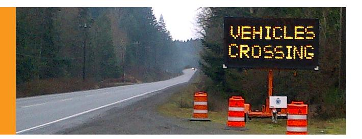
The BC Traffic Control Manual includes a number of traffic control devices beyond signs, cones and barriers that can help to mitigate traffic exposure risks.<sup>1</sup> When used in combination with other safety controls, these devices can reduce the risks of a worker being struck by a motor vehicle. There are also many other benefits:
